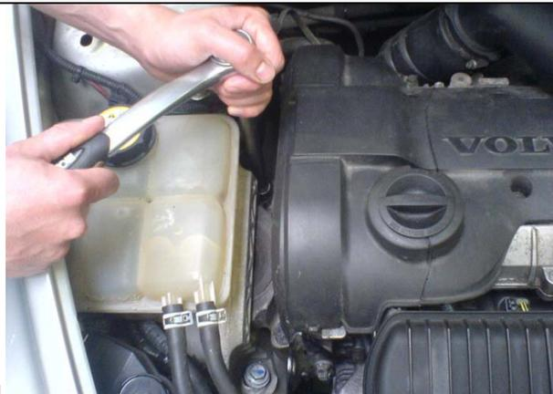
Remove the two bolts from the right hand side engine mounting. Remove the protective cover from under the engine. Put the lift jack under the oil pan and lift up the engine slightly, max 10mm. Push the engine backwards.
