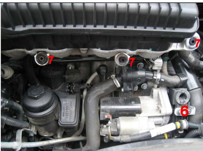
Assemble the plastic distance to the upper rubber holder(7).
