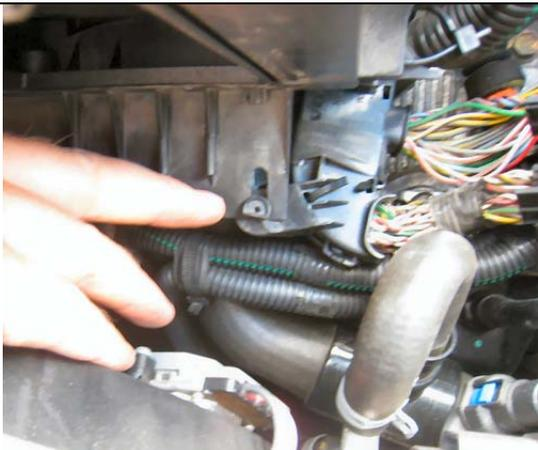
Turn the electrical harness and disconnect it from the air filter box.
