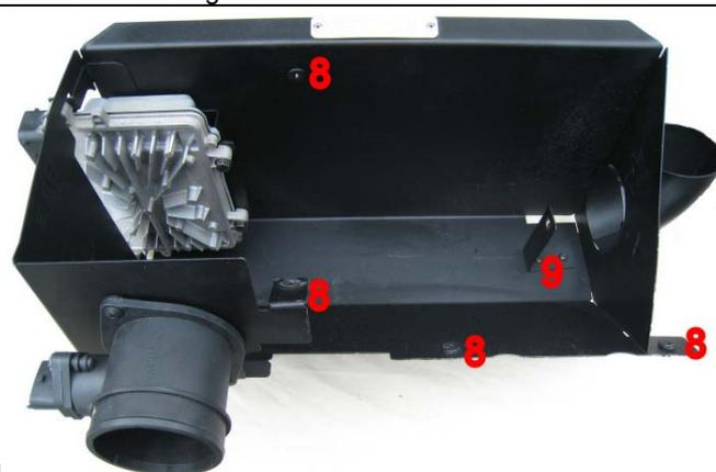
Assemble the 6 plastic clips to the plate (8). Assemble the MAS and the ECU to the plate . Assemble the rod (9). (as picture shows)
