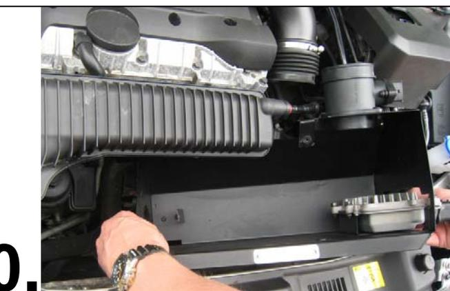
Assemble the plate. Push the plate down, make sure that the steering pin fits to the lower rubber holder (6) ← see picture 9.
