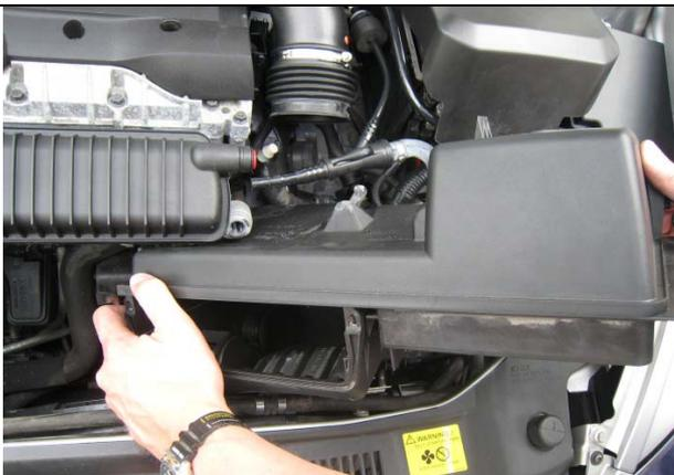
Pull the airfilter box straight up until lets go of the rubber holders. Then pull the box to the left and turn it at the same time upwards to release it.
