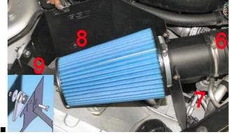
Mount the heat shield: Start with connecting the intake hose (6) to the pipe and the steering pin in the rubber lead-through (7). Mount the rod (8) with M6. (Do not tighten fully yet) Mount the rod (9) to the air filter before it connects to the Intake pipe and the chassis upper hold. Tighten all the loose screws (3), (8), (9).
