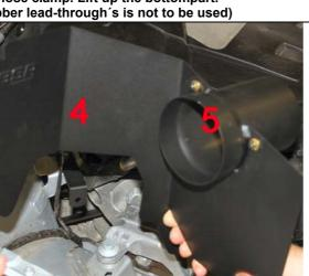
Mount the pipe (5) to the heat shield (4). Use M5.
